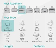
LS – Ledges on long side SS – Ledges on short side RP – Recessed post
